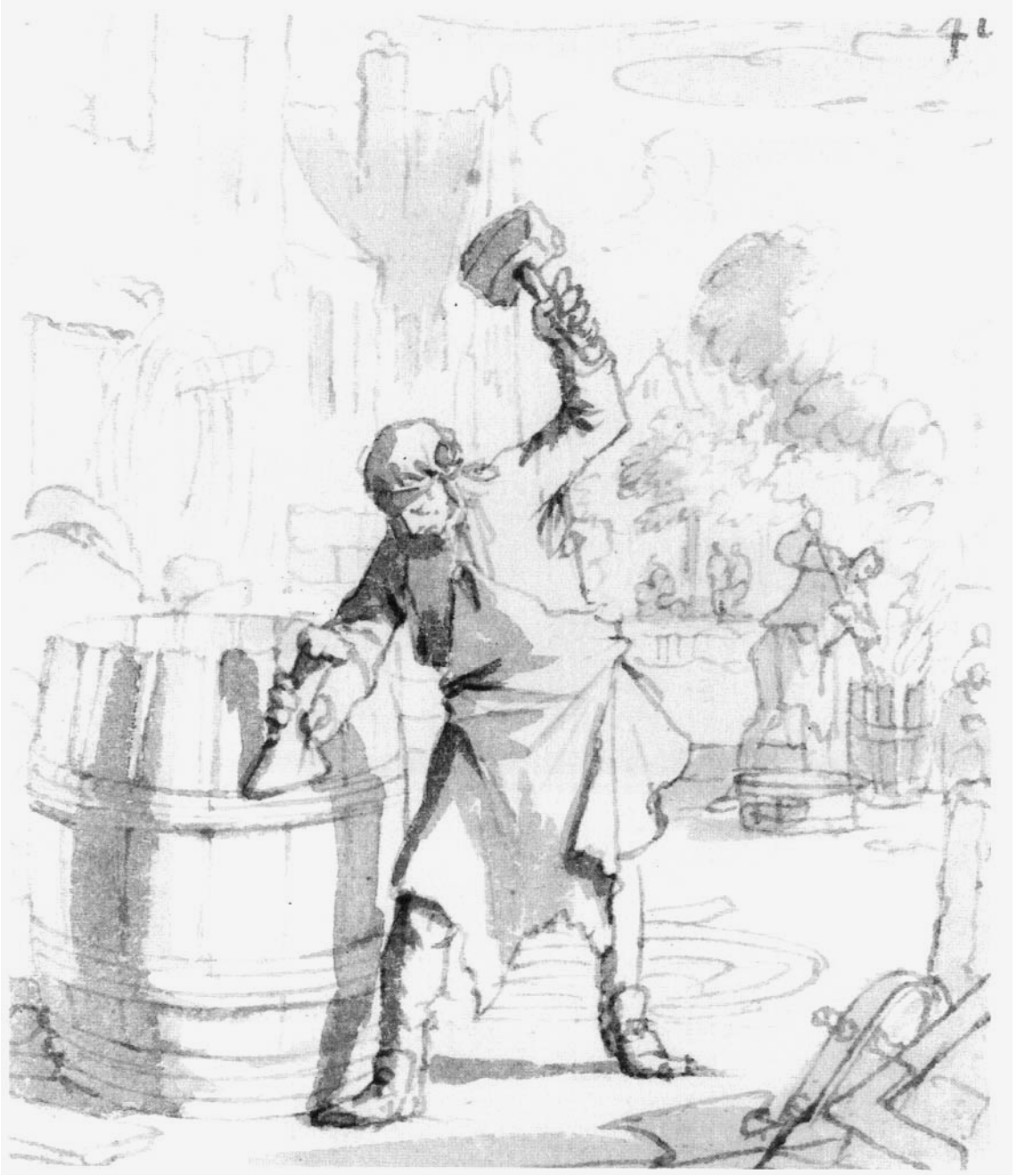
17. Jan Luyken, the cooper from Spiegel van het Menselyk Bedrijf , drawing, before 1694. The short poem in this case only says that cooperage produces positive results. The cooper is pounding hoops into place on a barrel while in the background a man is burning the inside of a nearly completed barrel. That would act both to seal the interior and also remove potential sources of impurities. Source: Source: Amsterdams Historisch Museum A13404
